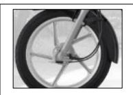
110 mm diameter Front and Rear Brake Drum
